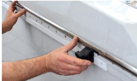
Place the fender profile and the fixing bar marking the right position of the steel bar with a felt-tip pen.
