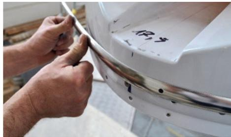
Drill holes in the boat using the same holes of the bars as a guide, point the track screws over the entire circumference boat.
