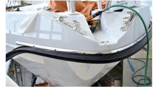
Apply one of the two base modules (the two base modules are perfectly the same), screwing the screws till when the profile stays on place.
