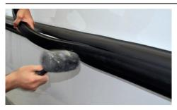
Apply the closing profile by pressing with a rubber hammer.
