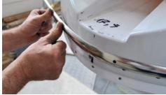
Drill holes in the boat using the same holes of the bars as a guide, point the track screws over the entire circumference boat.
