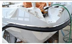
Apply one of the two base modules (the two base modules are perfectly the same), screwing the screws till when the profile stays on place.
