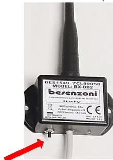
If the control unit is equipped with a radio wave remote control, the pairing procedure is the same as the infrared system, according to the installed model circuit board.
