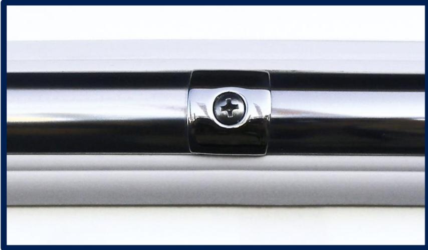
This small accessory designed for SPHAERA has multiple advantages. Its main purpose is to **fix the joining parts** to the boat **without having to drill extra anti-aesthetic holes**, moreover the so finished bars will keep their position perfectly and the **screws** will be all **equidistant**.
