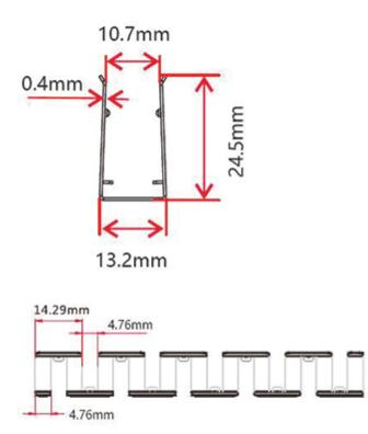
This profile can be mounted using screws in any gaps where the channel bends.
