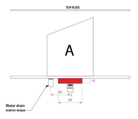
With this option, the encoder is assembled together with the actuator motor at the base of the pedestal. In order to keep the minimum and maximum heights of 340mm and 690mm, an additional protective housing must be installed underneath the pedestal in order to contain the working parts at the lowest support setting. The product is supplied complete with a water drain which accepts a Ø12mm (outside diameter) tube with a push-fit design. As standard, a 1.3m signal cable is included.
