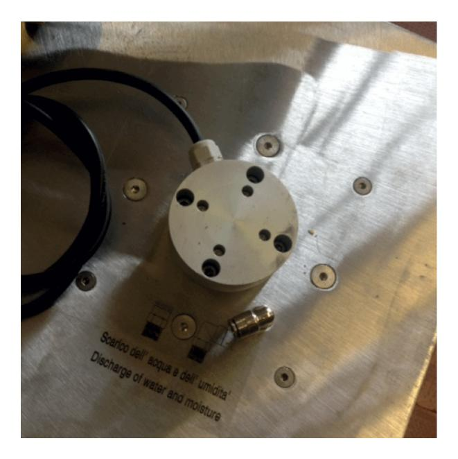
Example of encoder installation type 'B'
