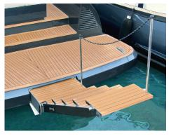
**Lightweight**Lascala weighs less than a hydraulic equivalent product thanks in the main part to the lack of a power pack. On average it weighs 30kg less than a traditional automatic ladder. In addition, there is a considerable space saving to be had by choosing **Lascala** once again thanks to the absence of a powerpack. The engine room can be more neatly packaged and more space potentially can be given to accommodation.
