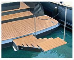
**Lightweight LaScala** weighs less than a hydraulic equivalent product thanks in the main part to the lack of a power pack. On average it weighs 30kg less than a traditional automatic ladder. In addition, there is a considerable space saving to be had by choosing **LaScala** once again thanks to the absence of a powerpack. The engine room can be more neatly packaged and more space potentially can be given to accommodation.
