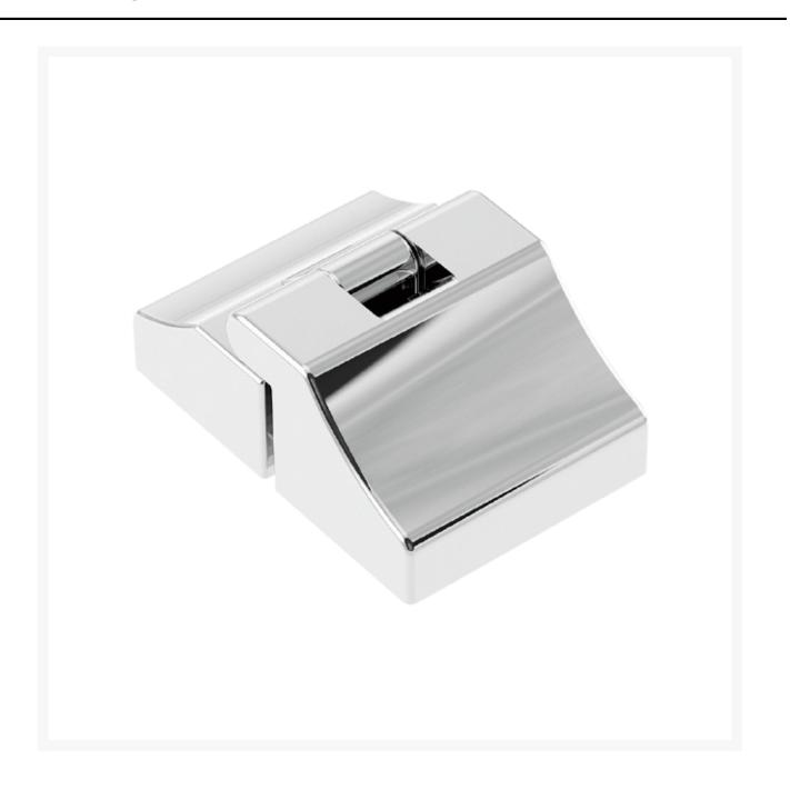
This 316-grade stainless steel hinge is of the highest possible quality. Machined from solid, and produced in small numbers, the hinge is not only high performing but is also beautifully crafted with a mirror polished finish. The hinge is fixed in place with 8 max. 4.5mm fixings and can operate through a 180° arc.
