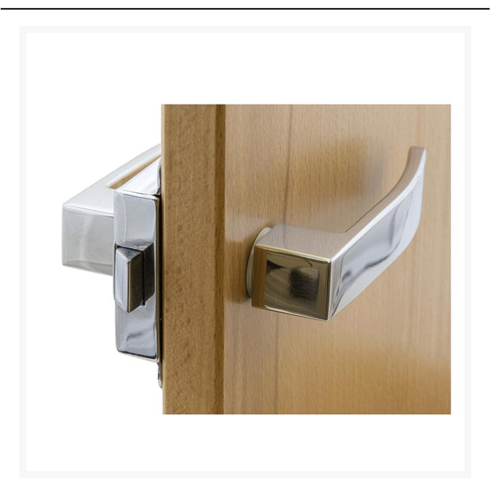
A rim latch lockset consisting of our 406100C rim latch, 850062 handles and 406800C striker. This lockset is enabled with a pin activated handle lock mechanism, making it ideal for use where a simple privacy function is required. The latch is a chrome-plated brass finish and has a universal door handing design.
