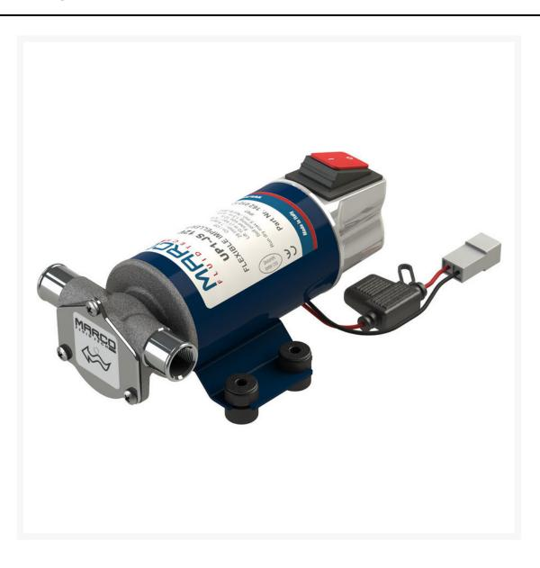
Self-priming electric water pump with self-lubricating NBR flexible impeller for prolonged service life and better performance. Nickel plated brass body with stainless steel shaft. Integrated ON/OFF switch for simple pump control.
