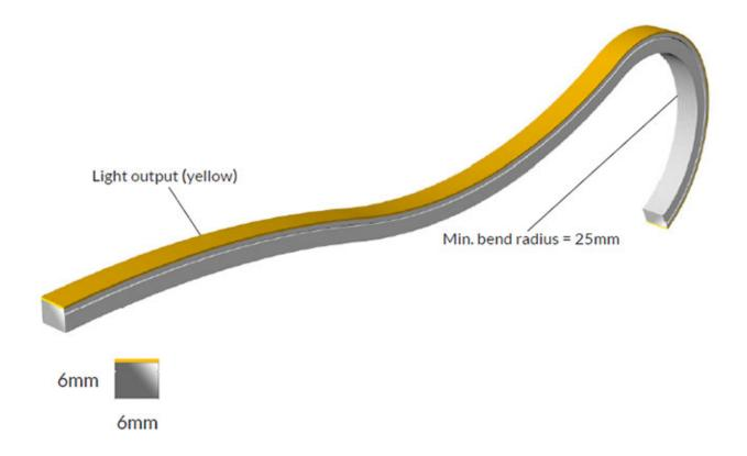
6x6mm Ultra-Mini Top View Neon Silicone construction IP67 Dimmable 12Vdc available on request Constant current version also available
