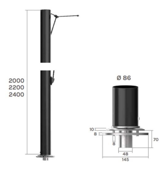
Pre-preg carbon fibre poles Storage bag included Clear UV protective coating Custom colour available on request Lightweight and strong Ø86mm pole system, Ø45mm and Ø66mm also available Internal pulley with Dyneema® rope and low friction rings Patented deck base with backing plate
