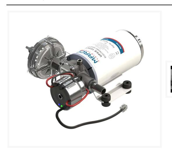
Self-priming automatic electric pump with helical PTFE gears, integrated check valve and electronic control. Nickel-plated brass body and stainless steel shaft. Main applications: fresh water pressure systems and shower kits, campers.
