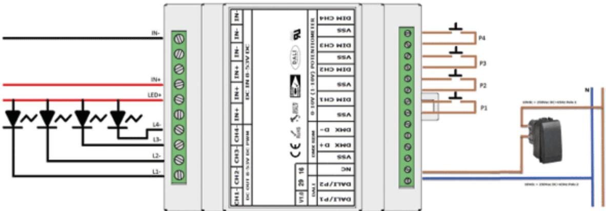
In this mode, the 4 output channels can be controlled using 4 independent switches as shown above.
