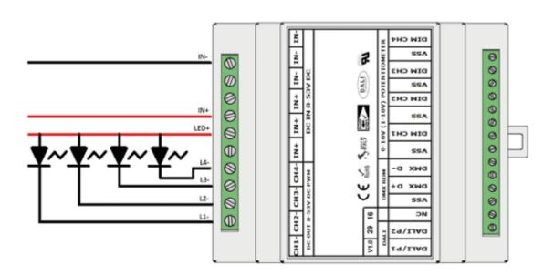
The 6012 dimmer module must be powered according to the polarity indicated above using the DC IN terminals (+ and -). In circumstances where the polarity is inverted, the device will not suffer any damage.
