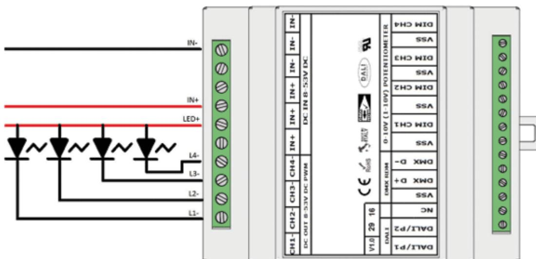
The 6012 dimmer module must be powered according to the polarity indicated above using the DC IN terminals (+ and -). In circumstances where the polarity is inverted, the device will not suffer any damage.
