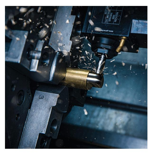
All Versari & Delmonte products are machined from solid. Using the latest CNC machining techniques, products are shaped from billet material, offering the ultimate in terms of strength, durability and finish. Working with both aluminium and 316-grade stainless steel, the items are suited to a wide range of applications.
