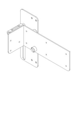
Steel bunk hinge mechanism with incorporated damper (left hand drawn)
