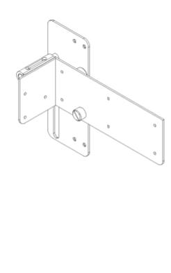
Steel bunk hinge mechanism with incorporated damper (left hand drawn)
