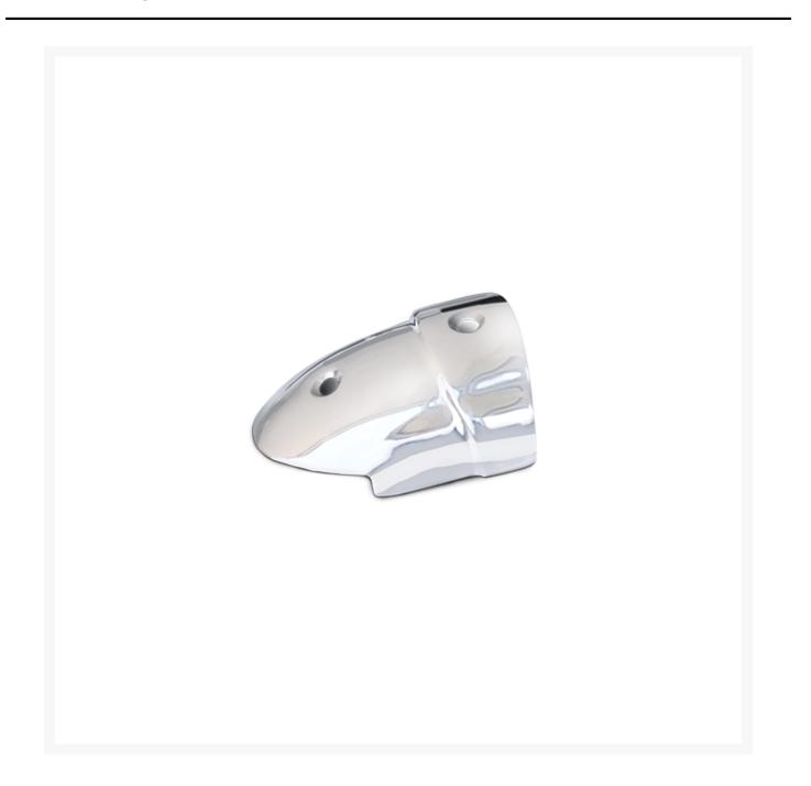
Cast 316 grade stainless steel end caps for use with Sphaera fender profiles. This particular end cap design is for use with Sphaera when fitted with standard PVC base only. The end cap is fixed in place with two screws. It is recommended to use a countersunk domed head 316 grade (A4) screw (not supplied).
