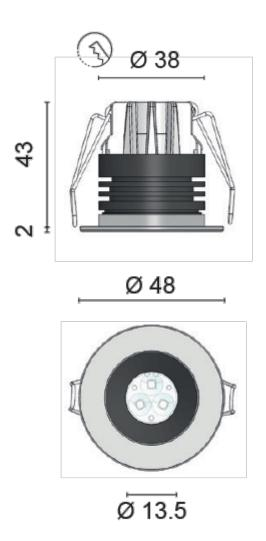
The Plutone spotlight has a deeper recess depth than other low voltage fittings in our range. This is caused in part by the anti-glare recessed light source, which sits deep within the light body, but also by the larger machined aluminium heat sink on the rear of the fitting. The size and performance of this heatsink has been carefully calculated in order to ensure that the LEDs operate at the optimal temperature for ultimate performance and longevity.
