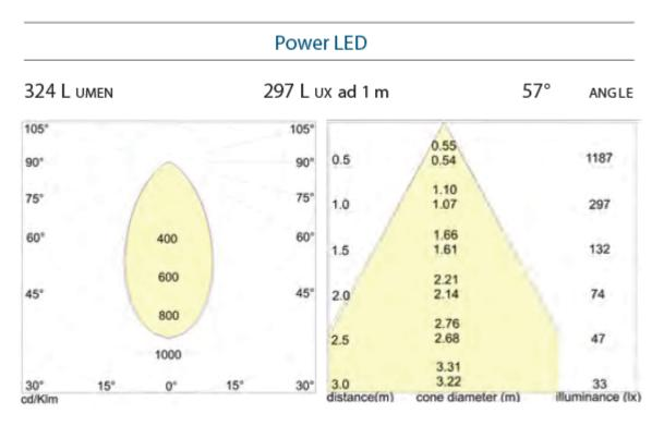
The photometric data in the ALHENA series is for a single module output.
