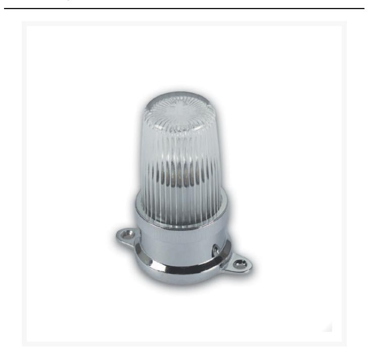
A pressure die cast brass white masthead anchor light, available in a polished brass and a chrome plated finish. RINA approved for boats upto 12m in length. Supplied with 12V 20W BA 15D bulb.
