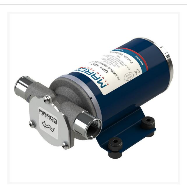
Self-priming electric water pumps with self-lubricating flexible impeller for prolonged service life and better performance. Nickel plated brass body with stainless steel shaft.
