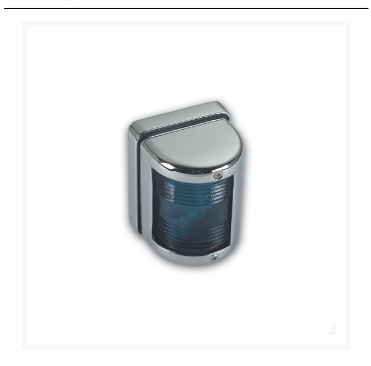
A pressure die cast brass green starboard navigation light, available in a polished brass and a chrome plated finish. Supplied with 12V 10W SV8 bulb. RINA approved for boats upto 12m in length.
