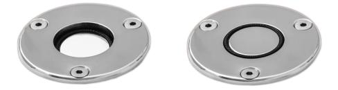
The innovative patented socket features a self-rising lid design. No need to screw and unscrew a lid, just simply push the pole straight into the socket and release with a spring loaded button installed on the base of the docked accessory. The socket also features a drain, allowing any water that enters to be sent straight to bilge.
