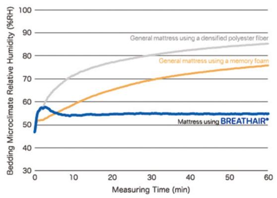
% Test Method : TOYOBO SKIN MODEL Method (Simulating the bedding microclimate during perspiration) Heating plate 37°C , Amount of moisture supply 120g/m<sup>2</sup>·s , Test environment 20°C x 65%RH
