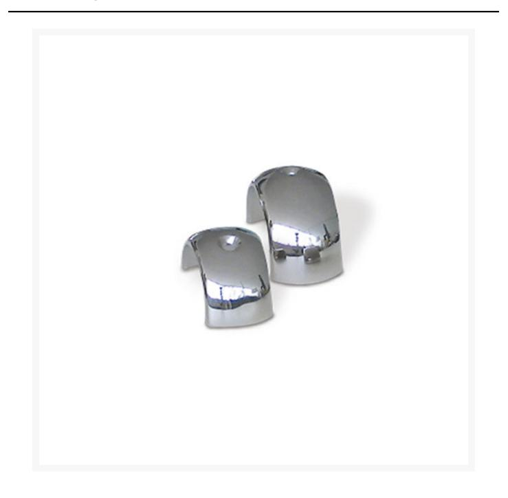
A cast 316 grade stainless steel joint cap for use with Radial 80. The joint cap is fixed in place with a screw. It is recommended to use a countersunk domed head 316 grade (A4) screw (not supplied).
